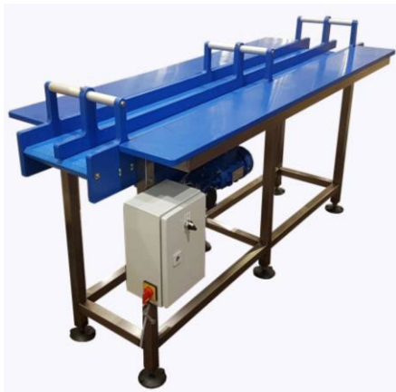
TWIN LANE CONVEYOR WITH MANUAL PACKING STATIONS
